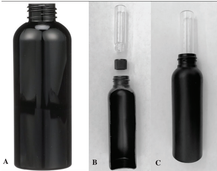
Figure 1. A. A low-cost 100 ml PET bottle can be used to construct a parasitoid emergence trap to study parasitism of MFC in the field. B. Basic components of the parasitoid emergence trap showing the PET bottle with modifications allowing for attachment to the tree branch and insertion of a glass collection vial. C. A fully assembled trap.
