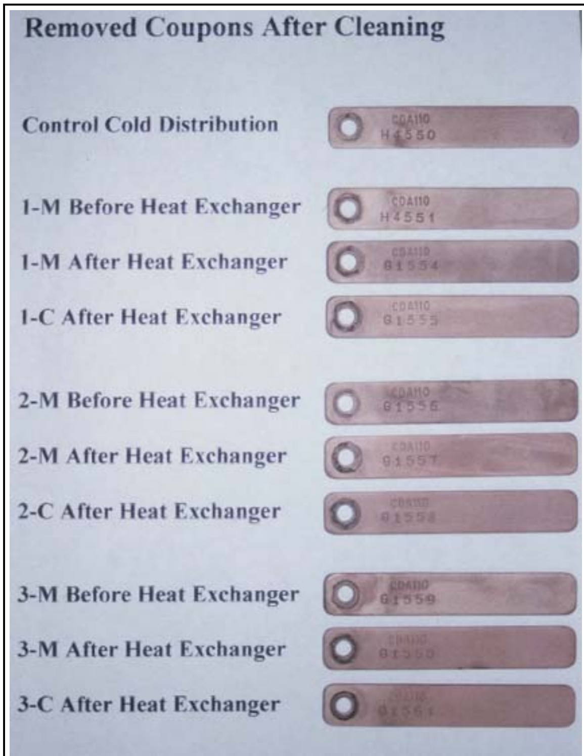
Figure 8. Corrosion coupons after cleaning.
