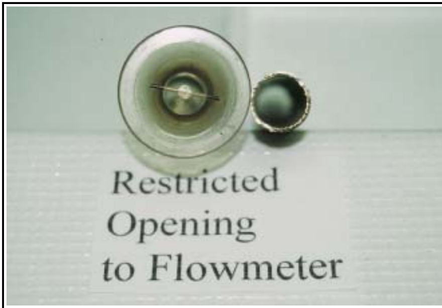
Figure 9. Restricted opening — flowmeter.
