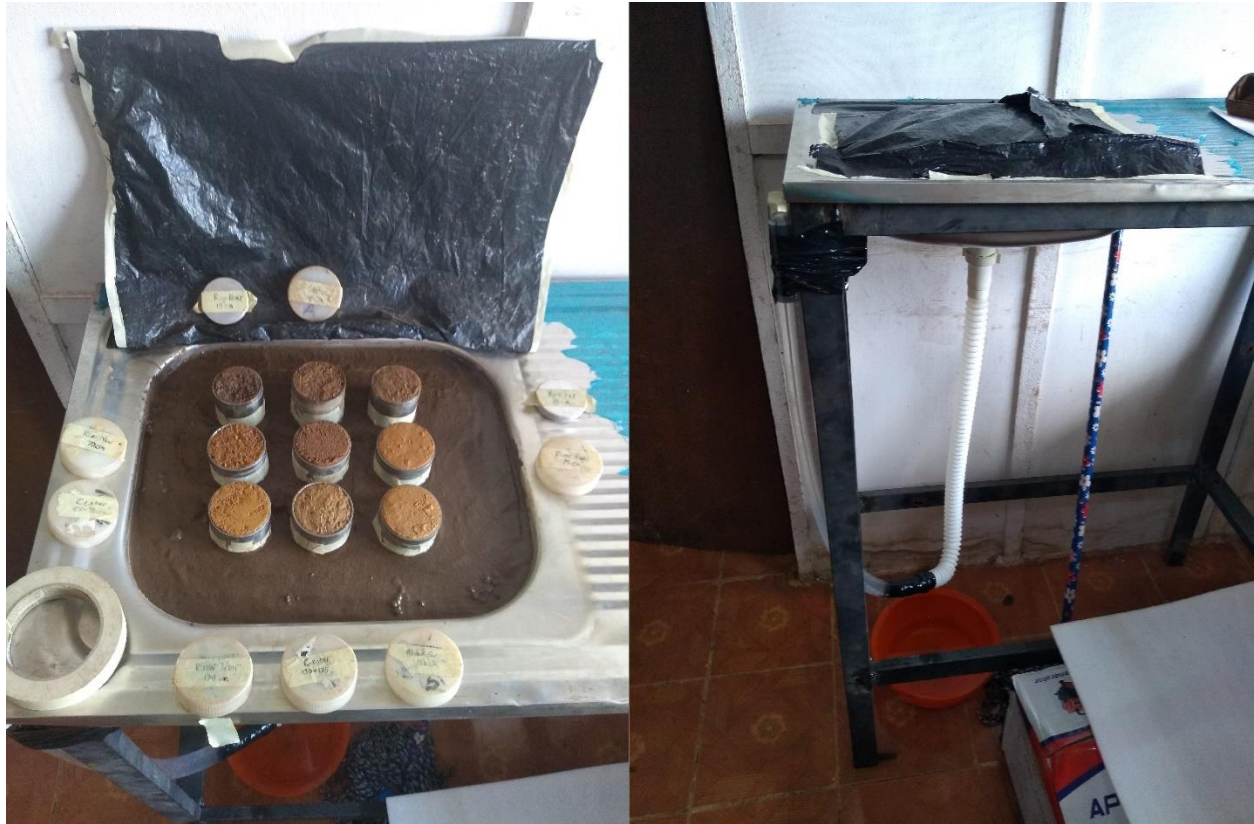
Figure 14. Sand suction table constructed from a standard sink. Soil samples shown on left.
