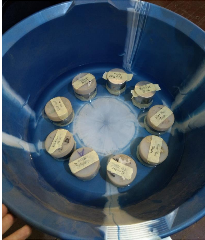
Water bath to saturate soil samples in preparation for measuring the soil water retention curve.
