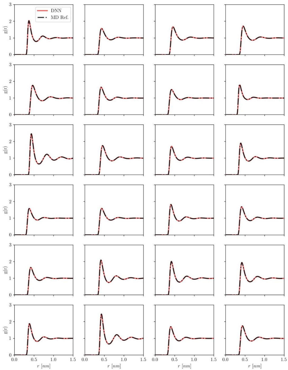
Figure A.10. Comparison between RDFs of DNN-based (solid red line) parameterized LJ potential and reference MD (dash-dot black line). Points are selected randomly from the dataset.
