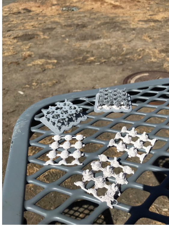
Figure 4.4 Failed attempt at 3D printing photonic crystals
