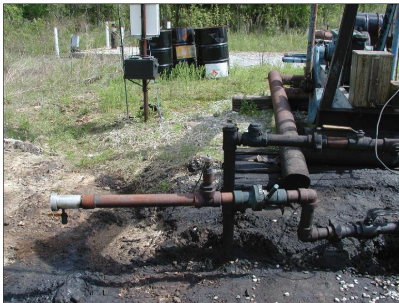
Figure 6 Gas prover (aluminum pipe on the far left) set up at an MGSC test site (Frailey et al. 2012c).
