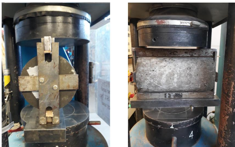
Figure 3.21: Set-up for tensile splitting strength test.
