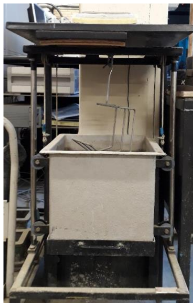
Figure 3.19: Equipment set-up for the determination of apparent weight of samples.
