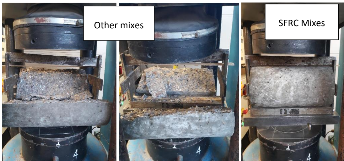
Figure 4.7: Failure mode of concrete cylinders of different mixes tested in tension.
