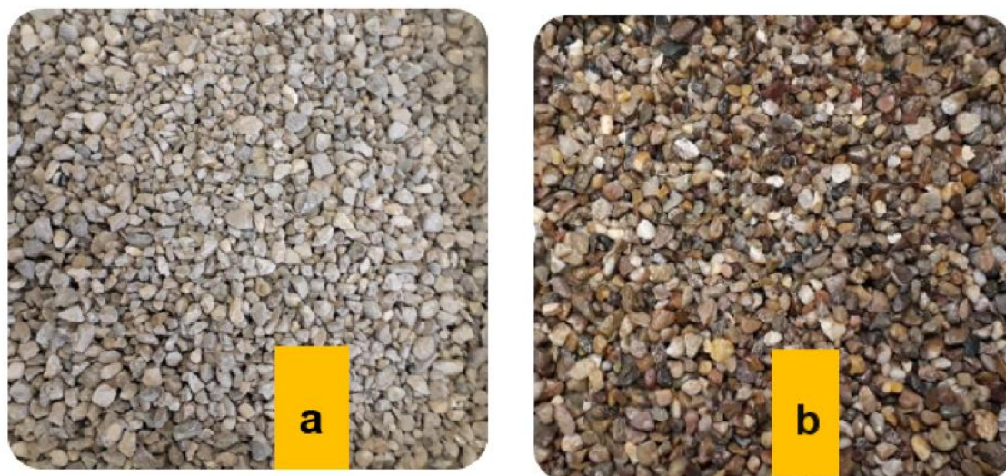
Figure 3.10: RCA before and after treatment for the removal of attached mortar.
