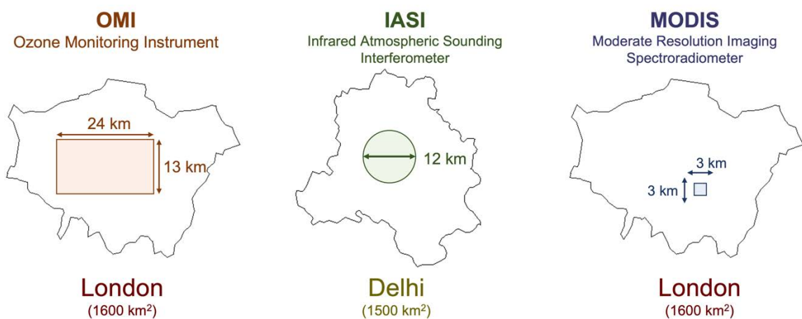
Figure 1.10 Schematic diagram showing the spatial resolution at nadir from different satellite sensors relative to size of the cities London and Delhi.
