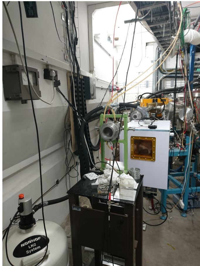
Figure 7.1: Setup at the MC40 Beamline, showing the coldbox (in white with an orange window) which can be moved via a motor mounted downstream of the proton beamline (which comes out of the silver coloured cylinder with a square hole). [111].
