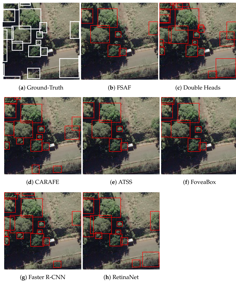
Figure 15. Tree detection with the top five methods, RetinaNet, and Faster R-CNN: performance in a challenging illumination scenario with shadows.
