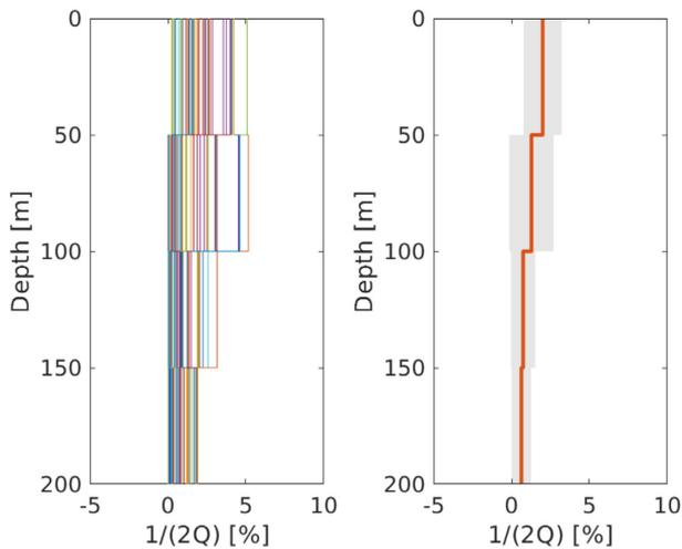
**Figure 12.** Damping profiles estimated with the up-down method at 44 sites of the G-network. Left: distribution of the 44 profiles. Right: mean (orange line) and spread ( $-\sigma$  to  $\sigma$ ) of damping values over the network. The mean  $Q$  values for the four depth intervals are—from top to bottom—25, 38, 76 and 87.
