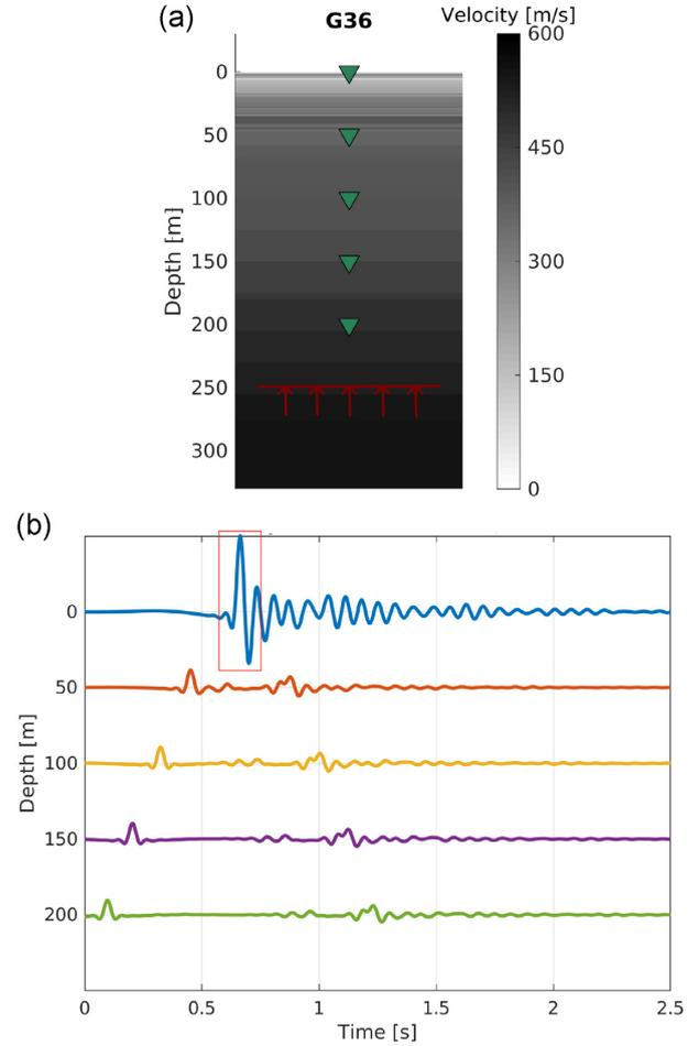
**Figure 3.** (a)  $S$ -wave model at borehole station G36, with five receiver levels (green triangles) and a plane-wave source at 250 m depth. (b) Elastic  $S$ -wave response at the five different receiver levels. The forward modelling is performed with a reflectivity code. A band-limited delta pulse ([2 20] Hz) is used as a source-time function. The red box shows the time window that is used to approximate the direct wave at the Earth's surface.
