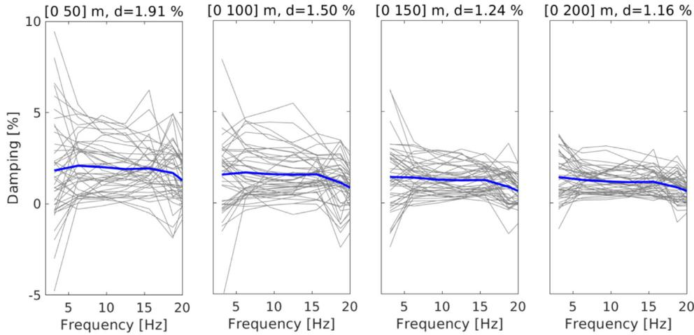
**Figure 16.** Estimated frequency-dependent damping (grey lines) for 44 sites over Groningen and the average over these sites (thick blue line). From left to right, the estimates are shown for the top 50, 100, 150 and 200 m, respectively.
