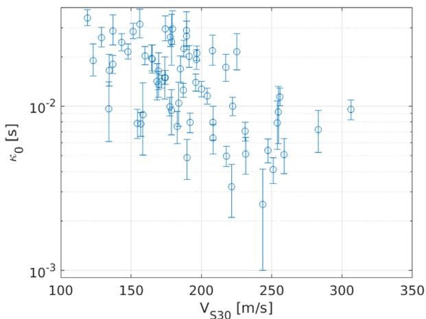
**Figure 15.** Estimated  $\kappa_0$  over the top 200 m plotted as function of  $S$ -wave velocity over the top 30 m. The circles depict the mean  $\kappa_0$  values for 63 sites. The error bars show the 68 per cent confidence interval (Appendix C).
