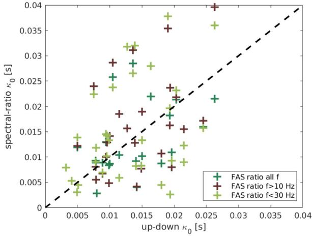
**Figure D1.** Cross-plot of  $\kappa_0$  values obtained with the up-down method and the spectral-ratio method, using different frequency bands. All frequencies means the entire frequency band with SNR > 3 dB. If the outcomes of the different methods were equal, they would lie on the dashed black line.
