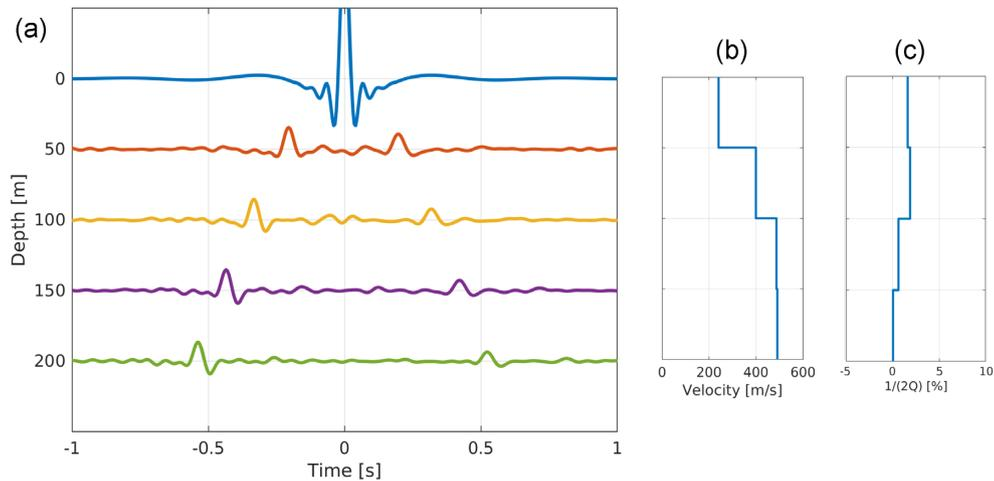
**Figure 11.** (a) The results of applying seismic interferometry by deconvolution at station G36 with a virtual source constructed at 0 m depth. The transverse-component result is shown in the band [2 20] Hz. (b) *S*-wave interval velocity model estimated from the timing of the upgoing wave in (a). (c) Damping interval model estimated from the amplitude differences between the up- and downgoing waves in (a).
