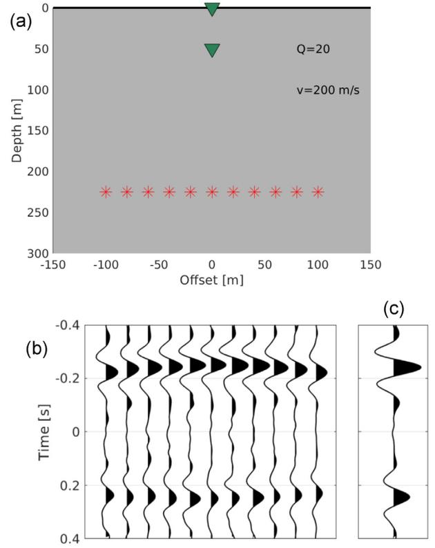
**Figure 6.** Numerical implementation of up-down method. (a) Configuration with an homogeneous subsurface, an array of sources (red stars) and two receivers (green triangles). (b) Deconvolution gather: the result of deconvolving the responses at the lower receiver with the ones at the upper receiver. (c) Result of stacking the deconvolutions over the sources.
