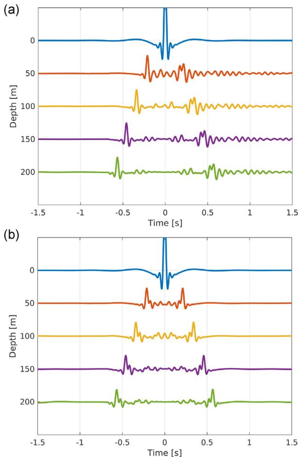
**Figure 4.** Responses retrieved with deconvolution (a) when an approximation of the direct wave recorded at the Earth's surface is used (as indicated with the red box in Fig. 3b) and (b) when the total response at the Earth's surface is used. In both cases, the complete forward modelled response, as shown in Fig. 3(b), is taken for the 50–200 m depth levels.
