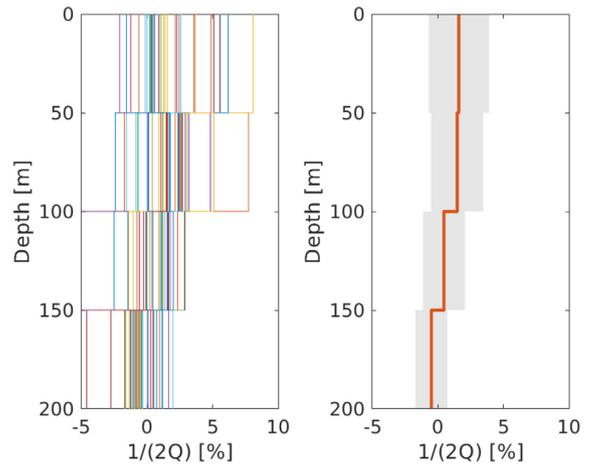
**Figure 9.** Damping profiles estimated with the upgoing method at 36 sites of the G-network. Left: distribution of the 36 profiles. Right: mean (orange line) and spread ( $-\sigma$  to  $\sigma$ ) of damping values over the network. The mean  $Q$  values for the four depth intervals are—from top to bottom—31, 34, 107 and  $-103$ .
