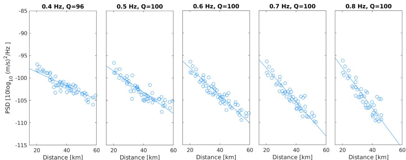
**Figure 18.** Recorded PSDs (circles) and fitted attenuation curves (lines) for five different frequencies. The recordings at 50 m depth are used. The  $Q$  values as estimated in the fitting procedure are shown above the curves. The PSDs are shown as function of distance from the active North-Sea coast, which is defined at the north side of the Wadden-Sea barrier islands, as an approximate west-east line 20 km north of the G-network.
