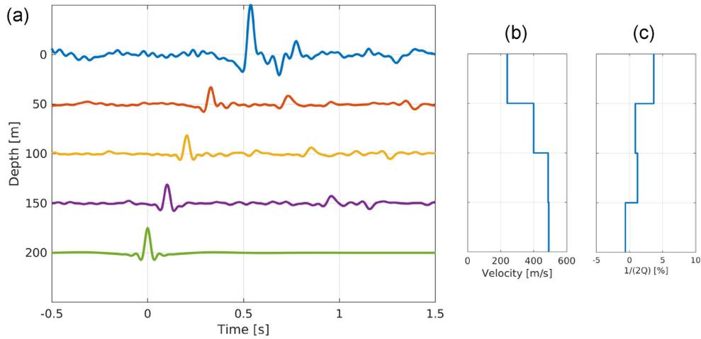
**Figure 8.** (a) The results of applying seismic interferometry by deconvolution at station G36 with a virtual source constructed at the 200 m depth level. The transverse-component result is shown in the band [2 20] Hz. (b)  $S$ -wave interval velocity model estimated from the timing of the upgoing wave in (a). (c) Damping interval model estimated from the amplitude decay of the upgoing wave in (a).
