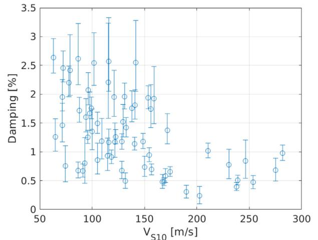
**Figure 13.** Estimated damping over the top 200 m plotted as function of *S*-wave velocity over the top 10 m. The circles depict the mean damping values for 63 sites. The error bars show the 68 per cent confidence interval (Appendix C).
