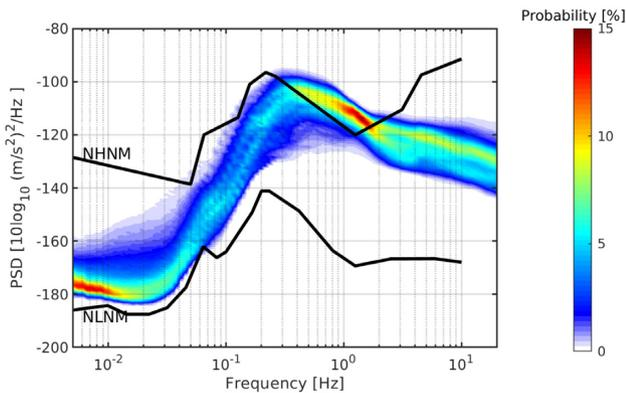
**Figure 17.** The vertical-component power-spectrum density distribution in 2020 at station G81B. For computing this distribution, the recipe in McNamara & Buland (2004) was followed. The measured distribution is compared with the new low noise model (NLNM) and new high noise model (NHNM) from Peterson (1993).
