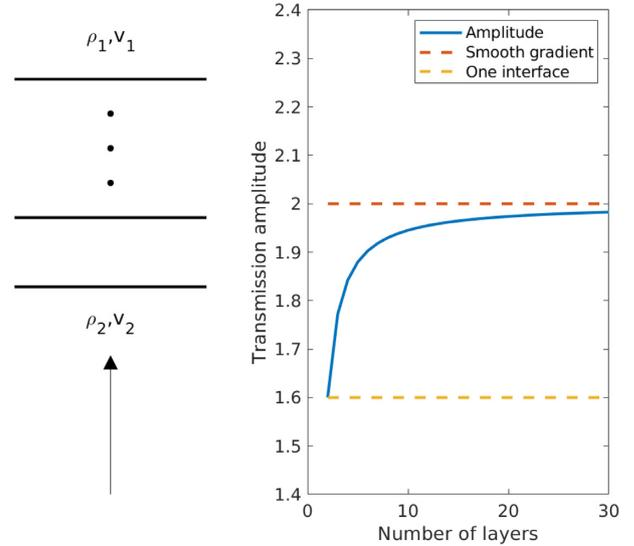
**Figure A1.** Left: a plane wave front with amplitude 1 impinges from below on a stack of layers and grows in amplitude due to reduction in impedance from depth level 2 to 1. Right: the transmitted amplitude above the stack of layers, as function of the amount of layers. It is assumed that the both the velocity and density are halved from depth level 2 to 1 and that the reduction in impedance occurs in equal steps from layer to layer.
