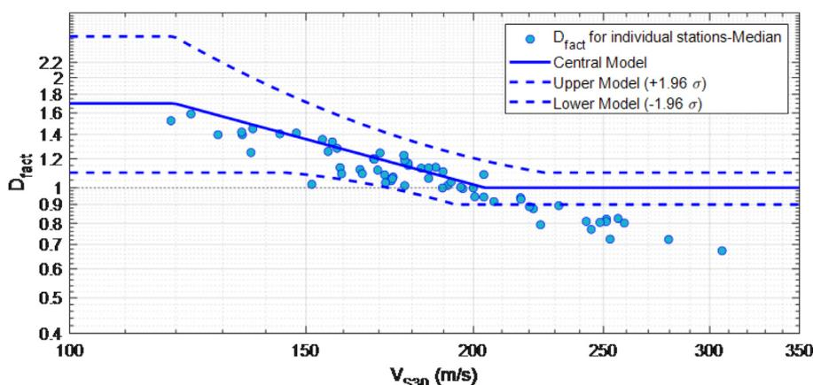
**Figure 19.** Estimates of  $D_{\text{fact}}$  for stations in the G-Network plotted against the  $V_{S30}$  for the station. The upper and lower models correspond to a 95 per cent uncertainty bound that consider uncertainty in each of the values of  $D_{\text{fact}}$  and uncertainty on the model fit.
