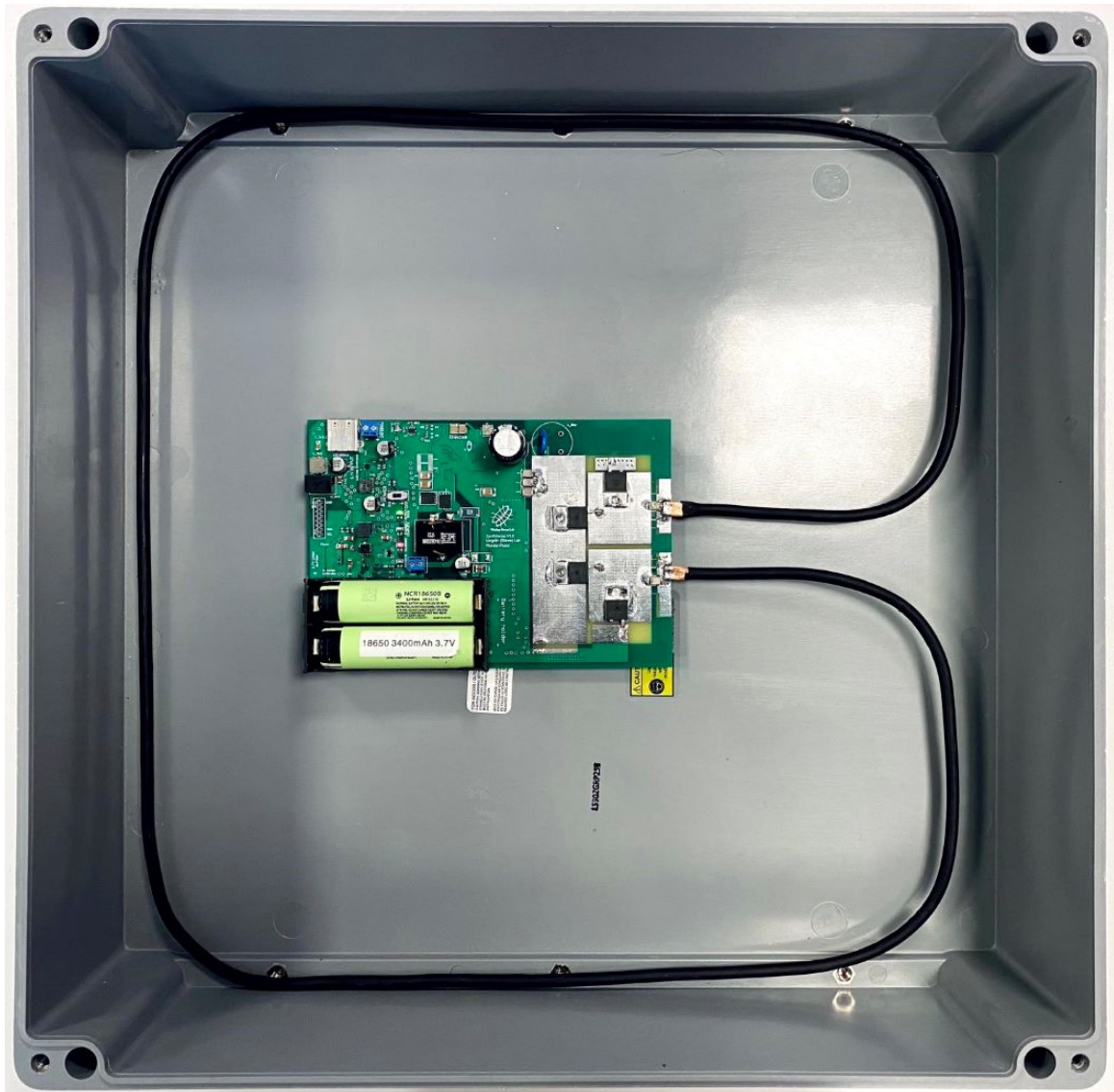
Figure 2.20: receiver side power electronics
