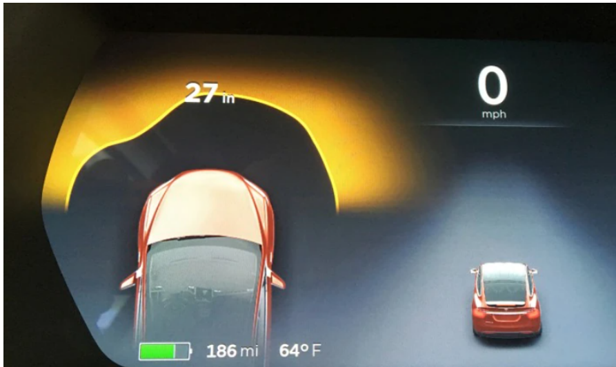
Figure 3.6: Automobile parking assist system based on ultrasonic sensors
