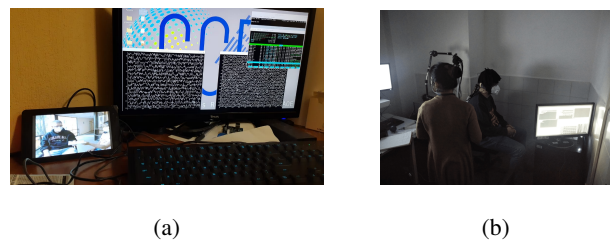
Fig. 3: (a) Raspberry running the PsychoPy based experiment (NeoGo screen) along with data acquisition of data streams simulating EEG and fNIRS signals (2nd screen only used for demonstration purposes). (b) Resting state test.
