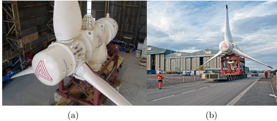
Figure 1.3: Photos courtesy of SIMEC Atlantis, showing the AR1500 turbine (a) inside the Nigg Energy Park warehouse during assembly and (b) en route to testing.
