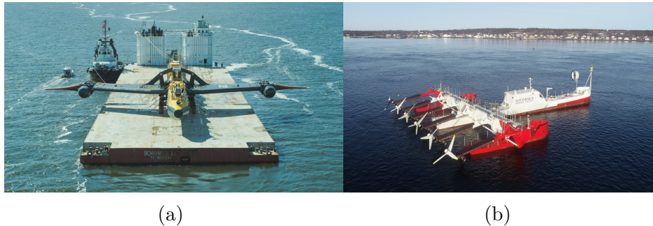
Figure 1.6: Examples of different floating tidal stream devices. (a) The installation of a barge-mounted dual-rotor O2 device, photo courtesy of Orbital Marine Power. (b) The first of the six-rotor PLAT-I 6.40 floating tidal energy platforms in the Pempa'q In-stream Tidal Energy Project, in the Bay of Fundy, Nova Scotia, Canada.
