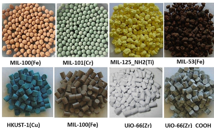
Figure 2.16: Frequently studied MOFs that have been shaped using granulation and pressing methods. Reproduced with permission from (Lee et al., 2021). Copyright 2021, Springer.
