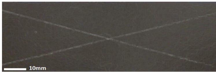
Fig. 7. Optical image of the cross-tube phantom with 200µm diameter
