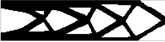
Figure 2.2: Optimized topology for 60 kN with the open filter.
