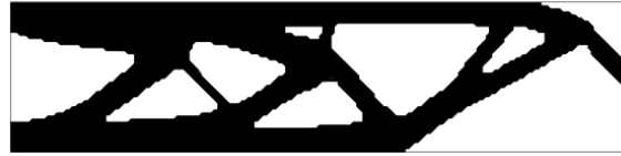
Figure 2.3: Optimized topology for 240 kN with the close filter.
