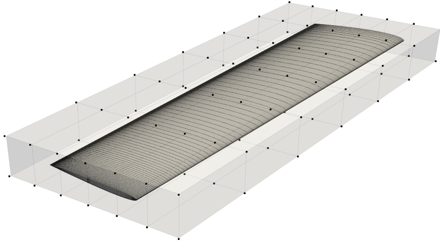
Figure 5.15: Initial wing geometry and FFD box.
