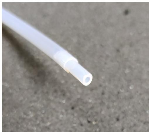
Figure 7.5 – The internal connector used to adjoin two lengths of PTFE tubing, reducing the internal diameter from 3mm to approximately 1.5mm
