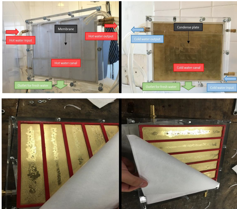
Figure 6.7. Working prototype for the desalinator design
