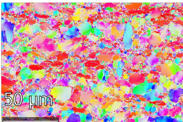
Figure 34: IPF-TD maps of rolled Ti-6Al-4V to 75% thickness reduction, at temperatures between 750 °C and 950 °C. Please note the difference in scale for 750 °C and 800 °C rolling.
