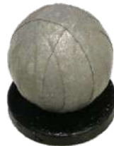
Figure 3.1: 14 mm spherical marker covered with reflective tape and mounted on a plastic base.
