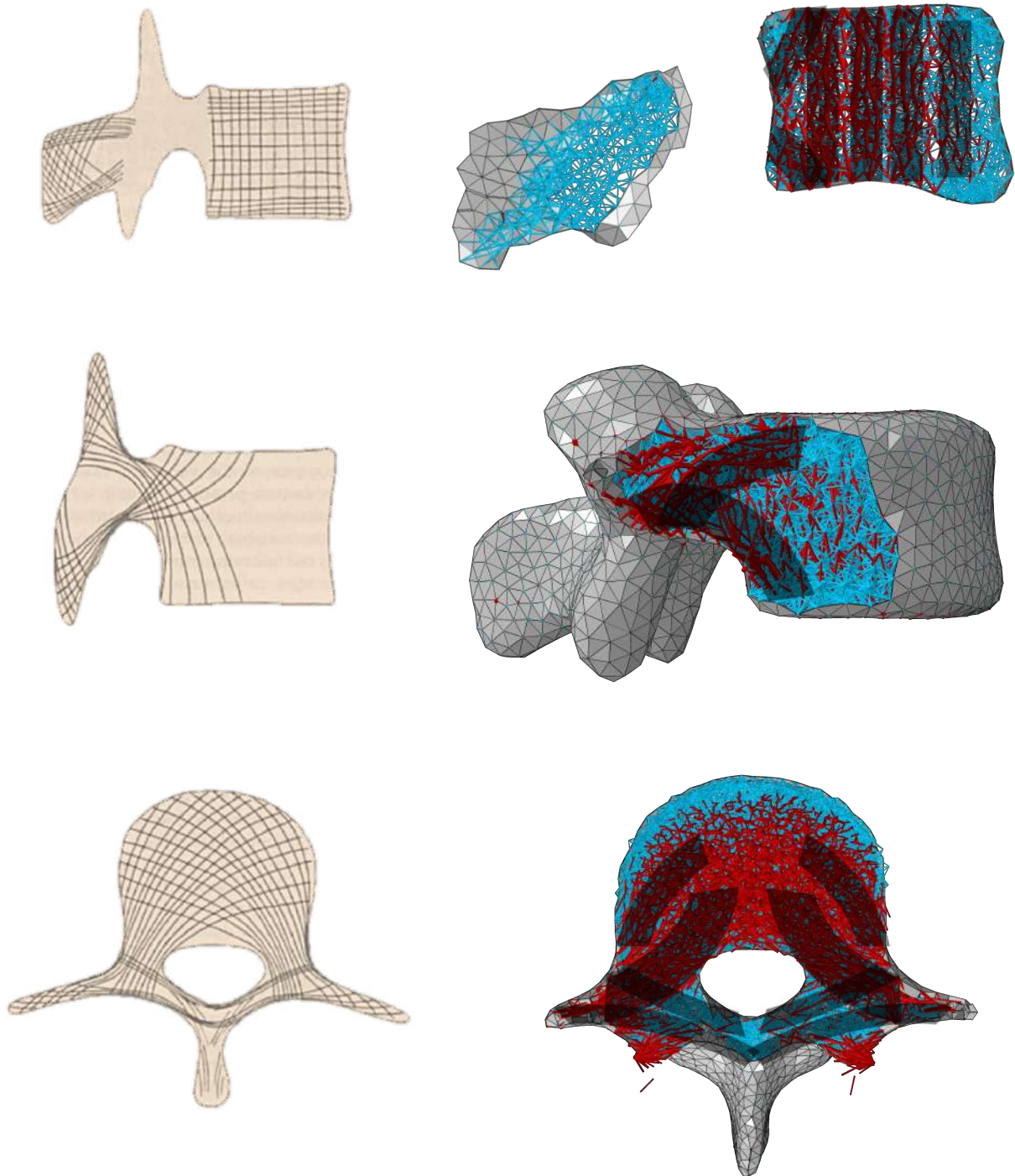
Figure 6.11: Structural architecture of the lumbar vertebra. On the left, observations made by Gallois & Japiot (1925). On the right, the converged L4 model adapted to 116 load cases representative of 18 daily living activities. Cortical shell elements are shown in grey. Trabecular truss elements with a radius of 0.1 \text{ mm} representing the ground matrix are shown in blue. Thicker truss elements are shown in red. Truss elements in the dead zone (with a radius of 1 \mu\text{m} ) are not shown for clarity.
