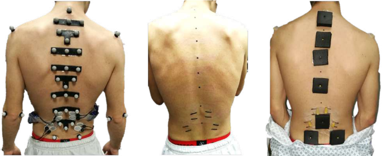
Figure 4.3: Reflective markers from the motion capture lab are replaced with cod liver oil capsules for the MRI scans. Left: Reflective markers and sEMG electrodes. Middle: marker and electrode positions marked with a surgical pen. Right: Cod liver oil capsules.
