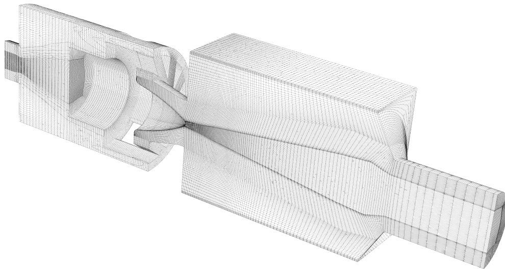
Figure 3.2: Vertical cut through the generated mesh consisting of 2.7 million grid points distributed over 144 blocks and refined in the premixing as well as the flame region. The combustion chamber has a 85 \times 85 \text{ mm}^2 cross section area and a length of 114 mm.
