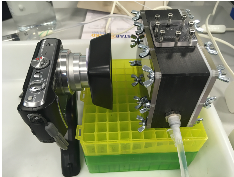
Figure 4.3: A photo of the experimental set-up consisting of a camera and the flow cell. The whole set up is kept in the dark whilst recording in order to block out stray light.
