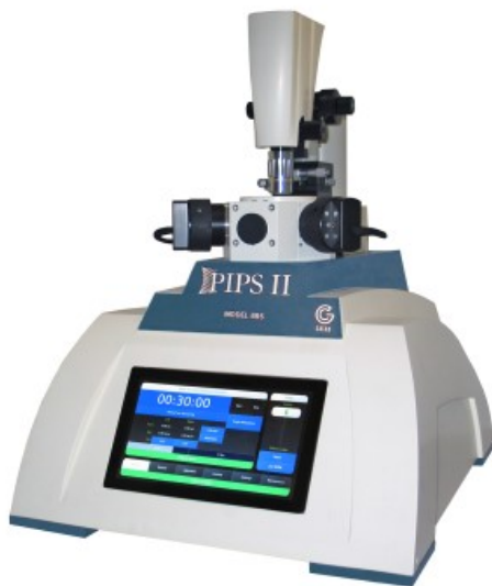
Figure 3.10: Facilities used for TEM observations (a) ion polishing system (“PIPS II System,” 2019) and (b) transmission electron microscopy (“FEI Tecnai F20,” 2019)
