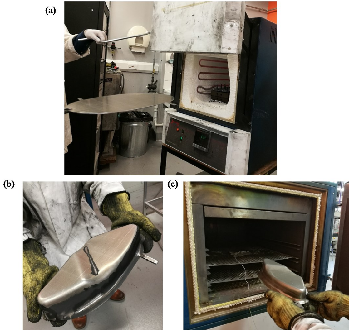
Fig. 6.24. (a) Blank heating in the furnace; (b) Example of a formed component; (c) Ageing of the formed component.
