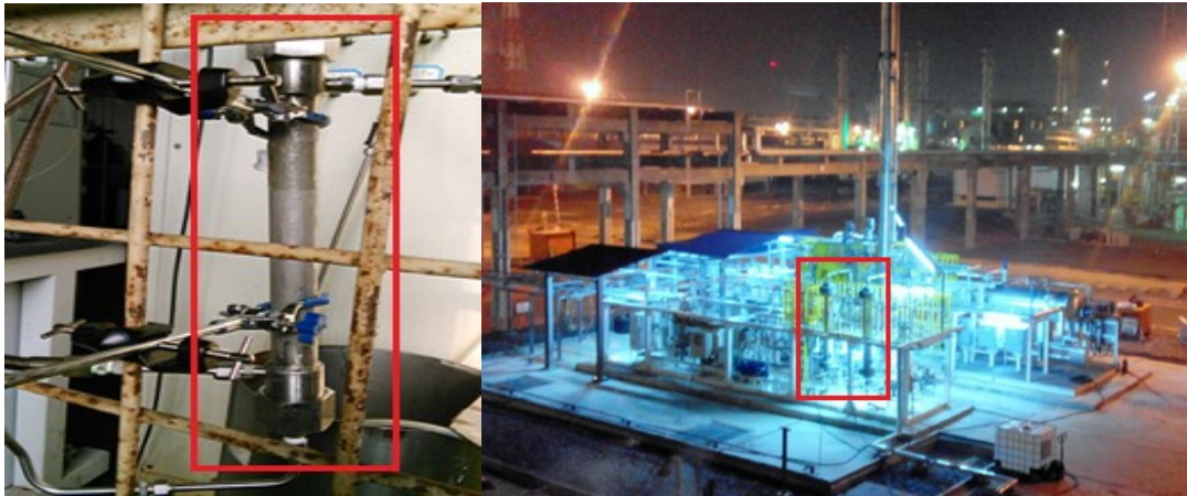
Figure 3.3: Vertical MBC operation. Left: lab scale MBC; Right: pilot scale MBC.
