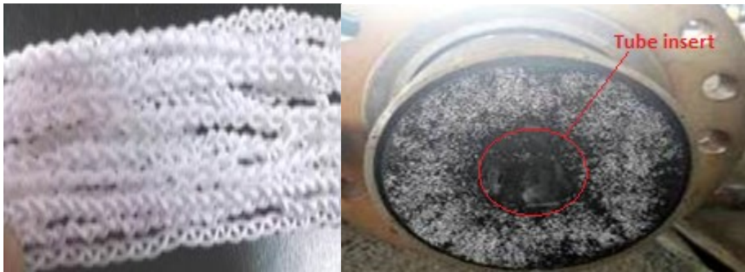
Figure 4.6: A: Braided HFM to increase the fiber length by 15% (i.e., from 2 to 2.3 m); B: cross-section of pilot-scale module with steel tube insert in the center to reduce the total membrane area.
