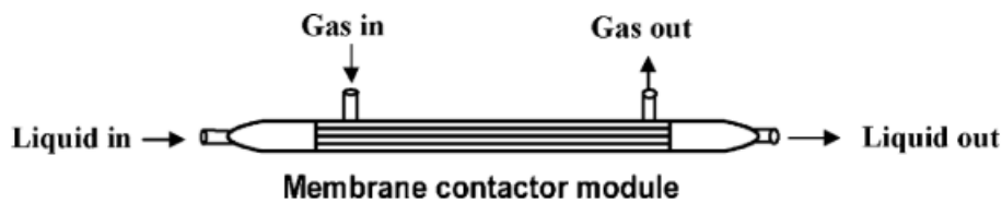
Figure 2.6: A parallel-flow hollow fiber MBC in co-current operation (Mansourizadeh and Ismail, 2009).
