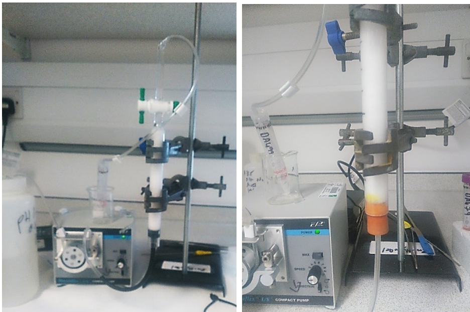
Figure 3.3. Photographs of the column experiment setup.
