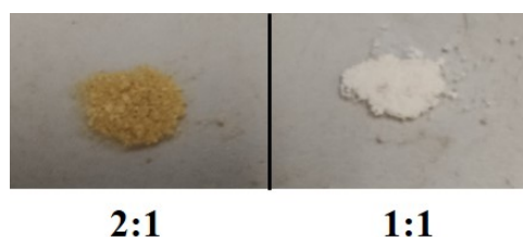
Figure 5-14: Images of the material afforded under evaporative crystallisation with stoichiometric ratios of 2:1 and 1:1 SA and AD.
