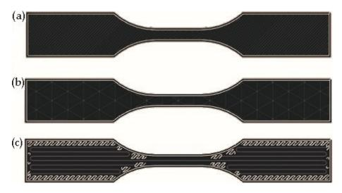
**Figure 5.** Sample preparation by CFF technology—sample marked "O" (**a**); sample marked "ON" (**b**); sample marked "C" (**c**)—blue lines indicate reinforcing carbon fiber, white lines indicate Onyx filament.
