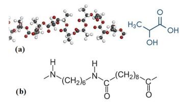
Figure 1. Structural model of: (a) PLA; (b) PA.
