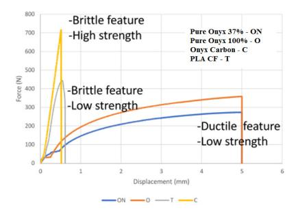
Figure 7. Tensile test results.
