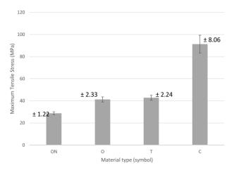
Figure 8. Average tensile strength.
