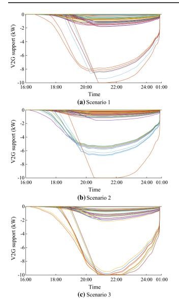
Fig. 7 PEV discharging power profiles for 10% PEV penetration rate.
