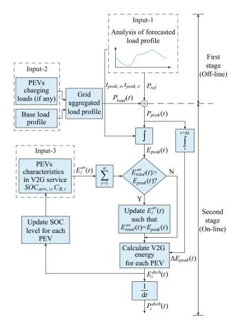
Fig. 3 Overall structure of V2G controller
