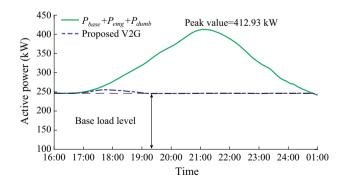
Fig. 8 Transformer loading profiles with V2G algorithm for 20% PEV penetration rate (scenario 3)
