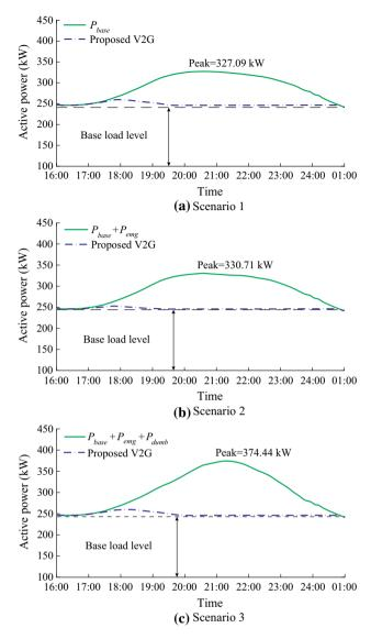
Fig. 6 Transformer loading profiles with V2G algorithm for 10% PEV penetration rate.
