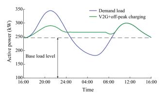
Fig. 9 Transformer loading profiles with V2G and off-peak charging algorithms for 5% PEV penetration rate (scenario 3)
