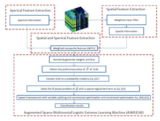
Fig. 1. The flowchart of proposed ASMLELM-WCFs framework.
