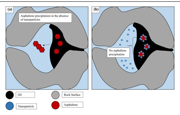
Fig. 4 Effect of nanoparticles in preventing asphaltene precipitation. a In the absence of nanoparticles. b In the presence of nanoparticles
