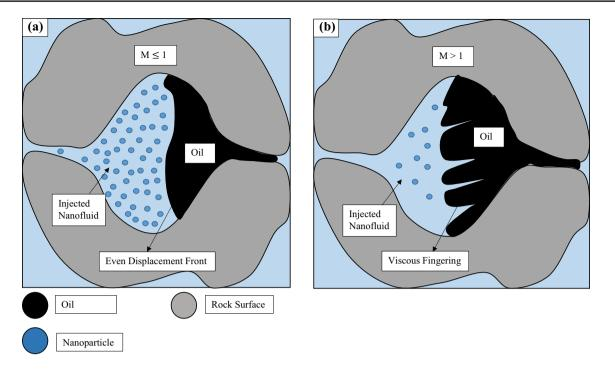
**Fig. 3** Effect of nanoparticle concentration on the viscosity of the injected fluid **a** highly concentrated nanofluid gives an even displacement front  $(M \le 1)$ . **b** Less concentrated nanofluid leads to an uneven displacement front (viscous fingering; M > 1)
