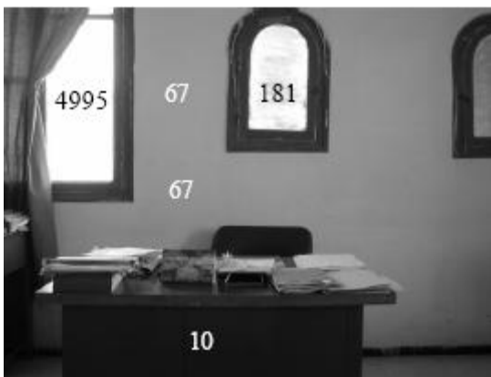
Fig.3 An example of a picture showing the values of the measured luminance in the macro-visual field
