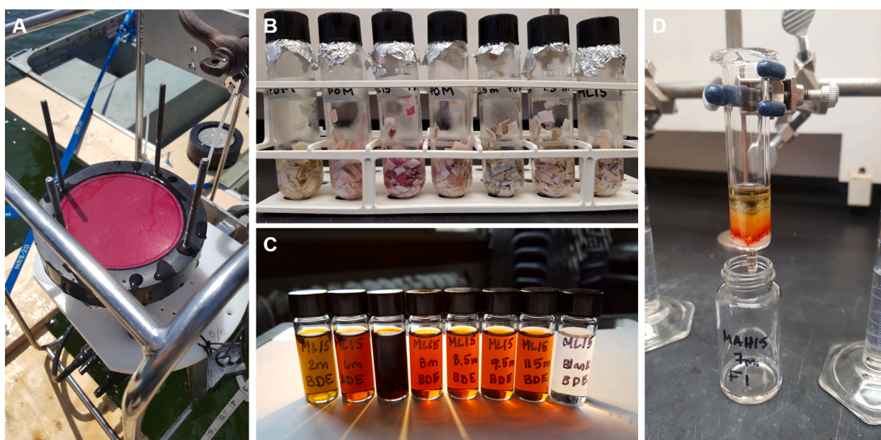
Fig. 2. (A) POM filter from the chemocline with abundant purple sulfur bacteria (PSB). (B) POM filters prepared for modified Bligh and Dyer extraction. (C) Bligh and Dyer extracts (BDEs) from POM filters. (D) Column chromatographic separation of the BDE from the PSB layer.
