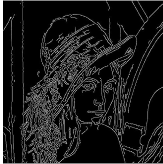
Figure 3: Edge Detected image using Canny method (Lena)
