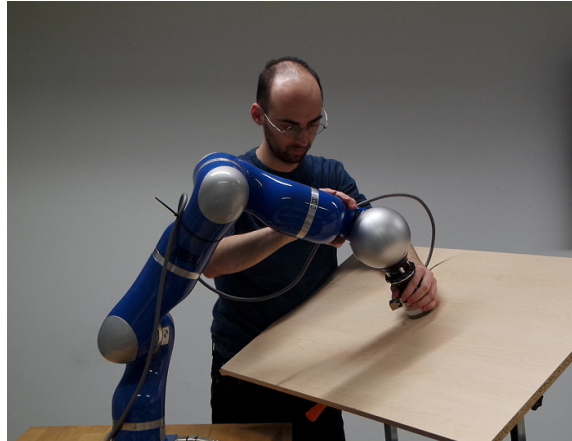
Figure 4.16: Demonstration of a circular wiping trajectory on a flat surface. The demonstration was repeated on surfaces of multiple orientations.
