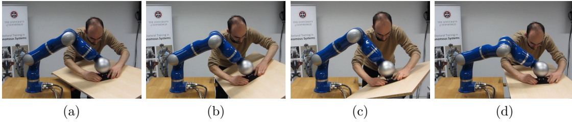
Figure 4.2: Example of using Programming by Demonstration for teaching a robot to execute circular wiping motions on a table, for a variety of different table positions and inclinations.
