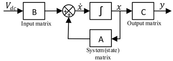
FIGURE 4. State-space vector diagram of a linear system.
