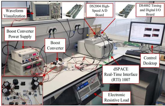
FIGURE 20. Test bench of the overall system.
