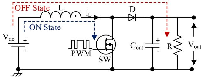
FIGURE 3. The block diagram of a boost converter.
