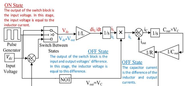
**FIGURE 6.** The differential equation model of the DBC.
