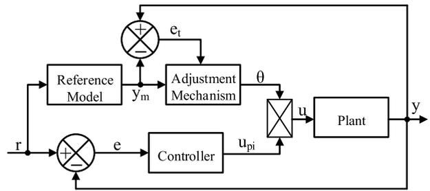
FIGURE 12. The block diagram of the MRAC.
