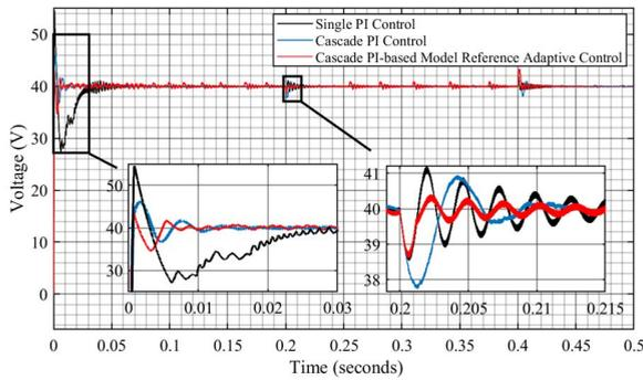
FIGURE 16. Comparison of control techniques under varying loads.
