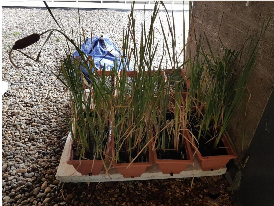
Figure 1. Wetland treatment microcosms (front) and pebble treatment microcosms (rear) atop a polystyrene base.
