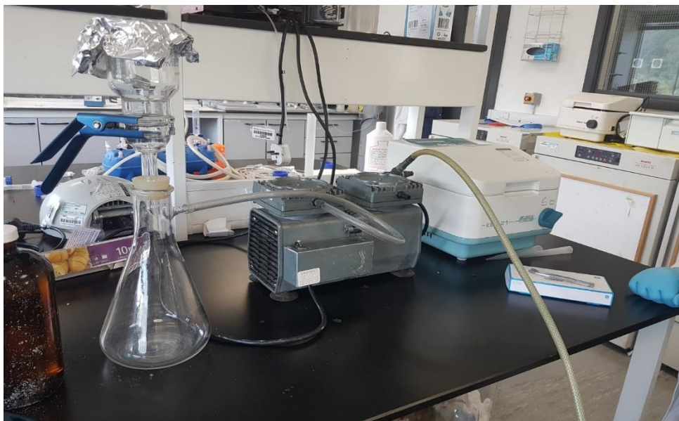
Figure 2. Filtration equipment setup, including electrical pump, MilliporeSigma™ Glass Vacuum Filter Holder and Büchner flask, rubber tubes, vice, tin foil cover, and 1L amber sample bottle.
