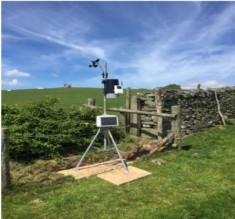
Plate 5.2 Unfenced free-draining stone wall (FD stone wall) adjacent to double fenced free-draining hedgerow (FD hedgerow). The weather station recorded rainfall, air temperature, wind direction and speed above the influence of either boundary type.
