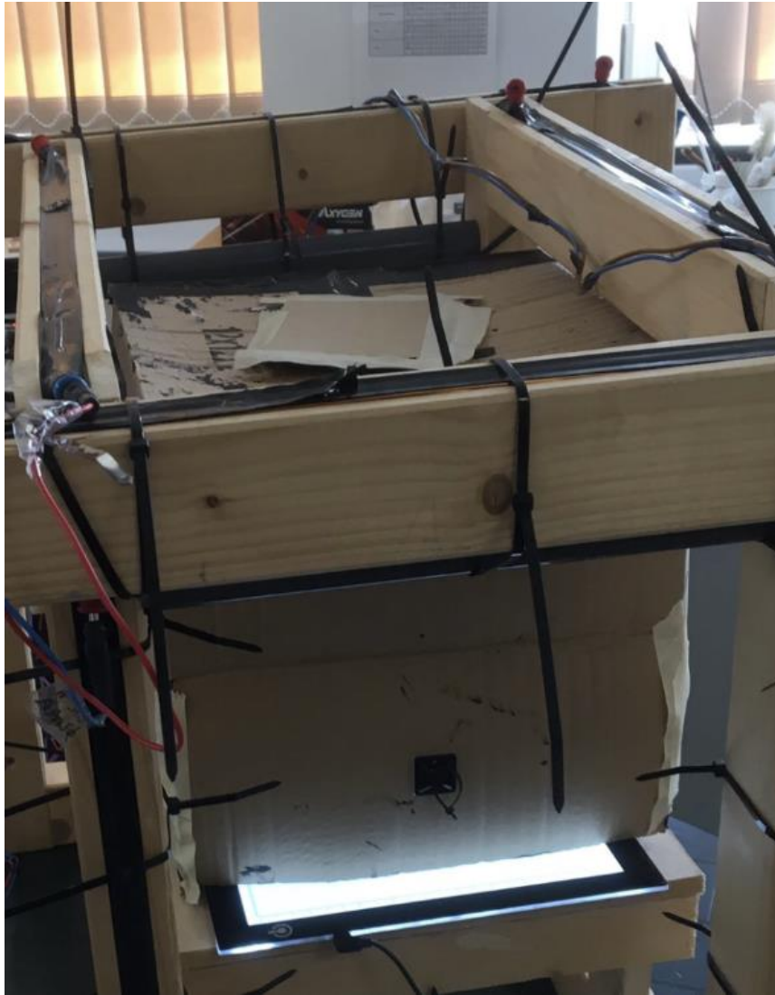
Figure 1: Photograph taken using a digital camera of the blackened cardboard box atop the illuminated drawing table (within a Helmholtz Coil) used during experiment 2.4.
