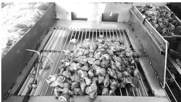
Figure 7.1. The whelk riddle used on Vagabond DO180 in the Isle of Man.
