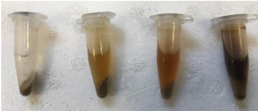
Figure S2. Image to demonstrate colour produced in supernatant from extraction of the Cambisol with different extractants. From left to right: deionised water; 0.5 M Na-citrate; 0.1 M Na-pyrophosphate; 0.5 M NaOH.
