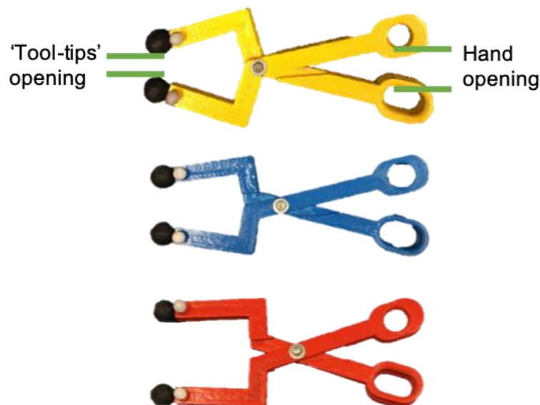
Figure 2.4. The three tools used in most experiments. The handles are on the right side. The motion capture markers can be seen near the black balls.
