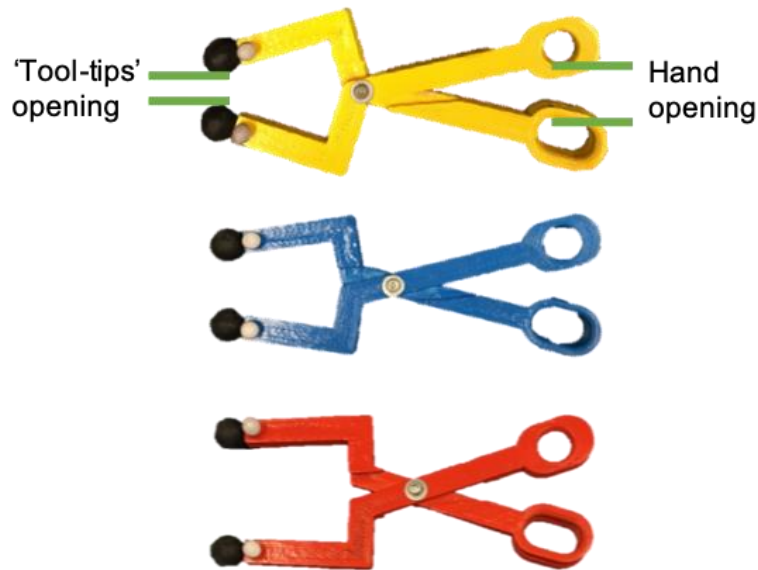
Figure 3.2. Pictures of the three pliers-like tools (same as Fig. 2.4). The yellow tool has a ratio of 0.7:1 between hand opening and tool-tips opening. The blue tool has a ratio of 1:1 and the red tool has a ratio of 1.4:1.
