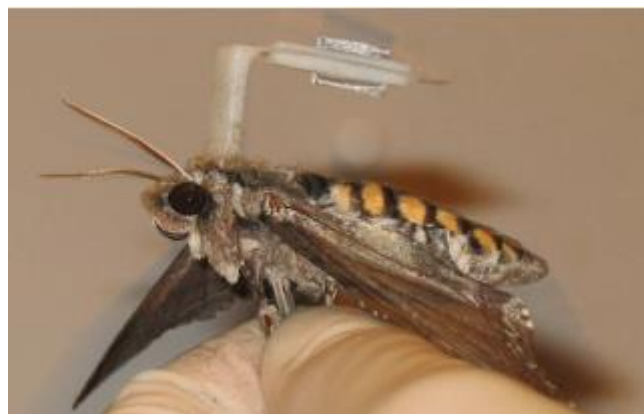
Figure 1.10: Fabricated energy harvester attached to Manduca Sexta [112].
