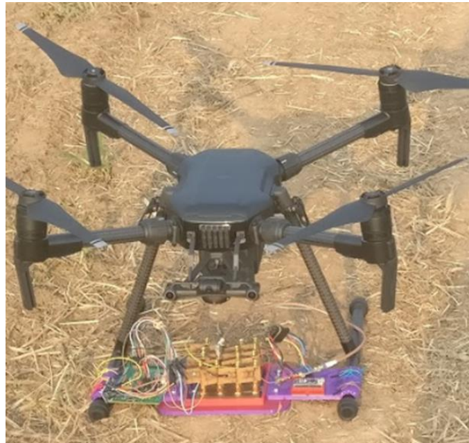
Fig 5.1: 3D printed housing unit for AoA system with integration of components to 3D printed unit
