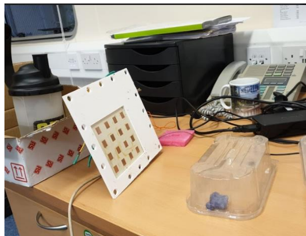
Fig 5.10: Experimental set up of antenna system and receiver placed 1m away from tagged bee inside box and antenna scanned from -50^\circ to 50^\circ in azimuth and elevation
