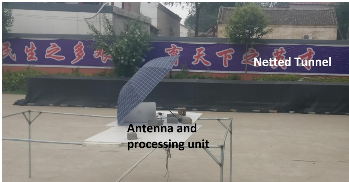
Fig 4.9: Constructed netted tunnel to house tagged bees during experiment and experimental set up of the receiver system
