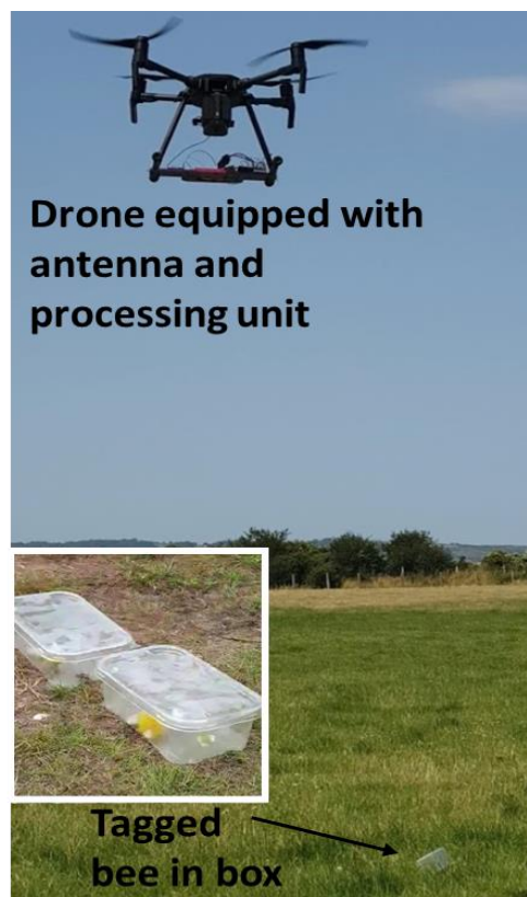
Fig 5.26: Experiment to test long-range bee tracking capabilities of autonomous system
