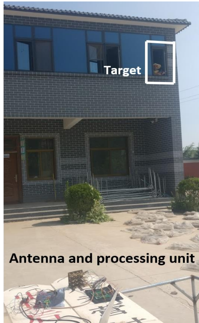
Fig 4.8: Experimental set up of testing 2D scanning capability of the system
