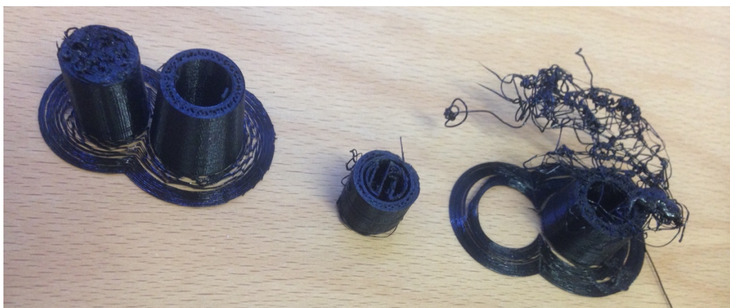
Figure 34: Early experiments with 3D printing, showing different densities and lattice structures.
