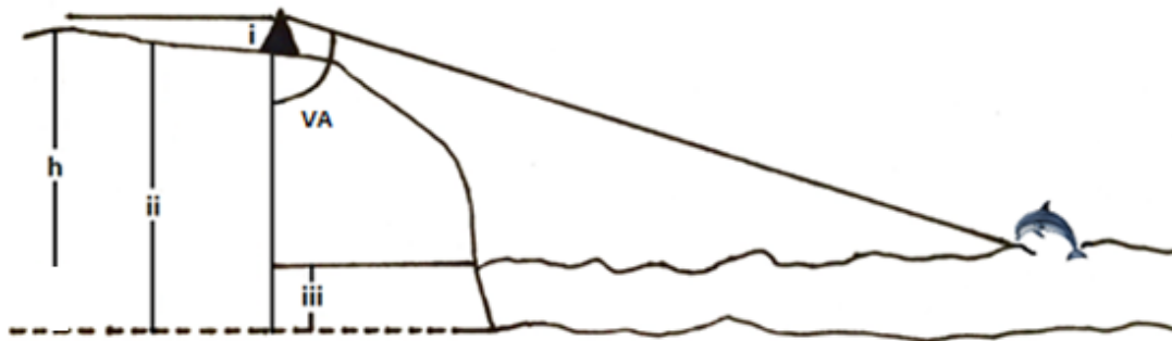
Figure 4.2 The angle and distances used to calculate the position of a marine mammal using a theodolite. (i) theodolite height, (ii) height of the survey site, (iii) tidal height, (h) theodolite height above the current sea level, (VA) vertical angle.
