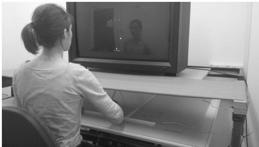
11 Figure 1. Experiment 1. The task was a target-directed aiming movement, performed using a handheld 12 stylus on a digitising tablet whereby the X/Y movement of the stylus on the tablet plane corresponded
