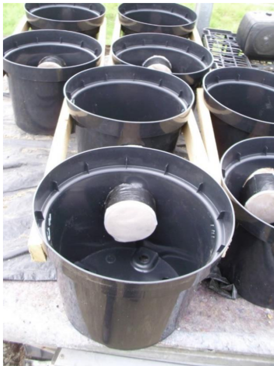
Plate 14: Interconnecting tubing was each filled with 2kg of sand and 20g of bone-meal, then the ends were covered n 40 micron screen
