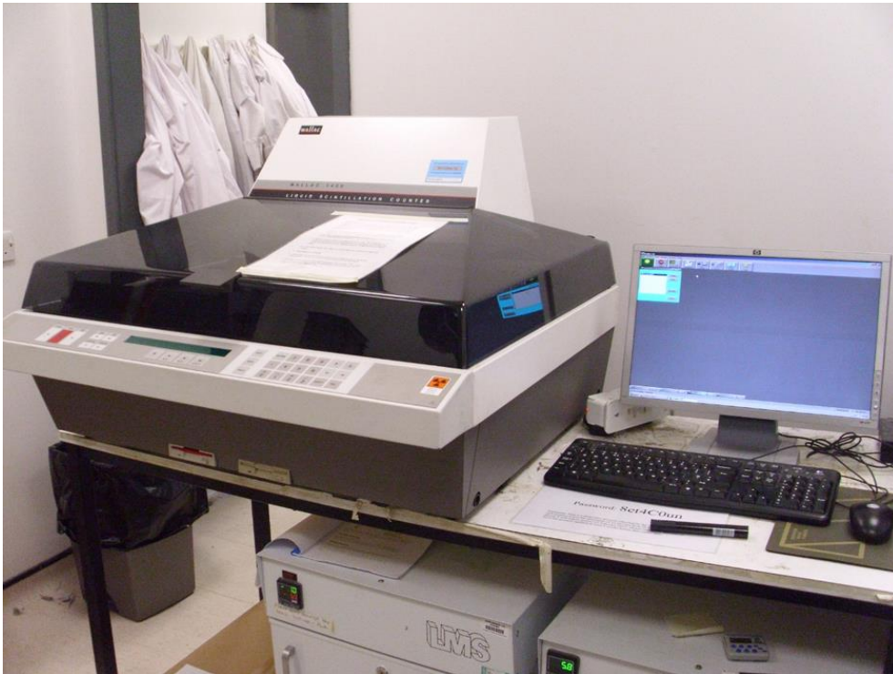
Plate 2: Wallac 1409 liquid scintillation counter located in the counting room and utilised for all ^{14}\text{C} analysis of vegetative, soil sand and liquid samples (Wallac EGandG, Milton Keynes, UK).
