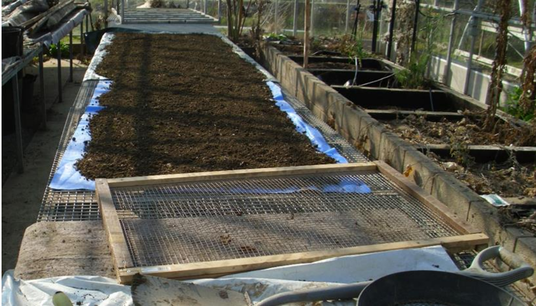
Plate 5: Soil removed from BangorDIVERSE was air dried before being passed through a 2 mm. sieve and utilised in the mesocosm experiments (Chapter3, 4 and 5).
