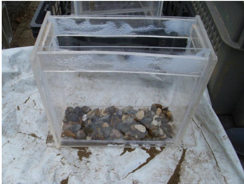
Plate 10: stones were placed in the bottom of the slabs to allow drainage and prevent anaerobic conditions from damaging the roots
