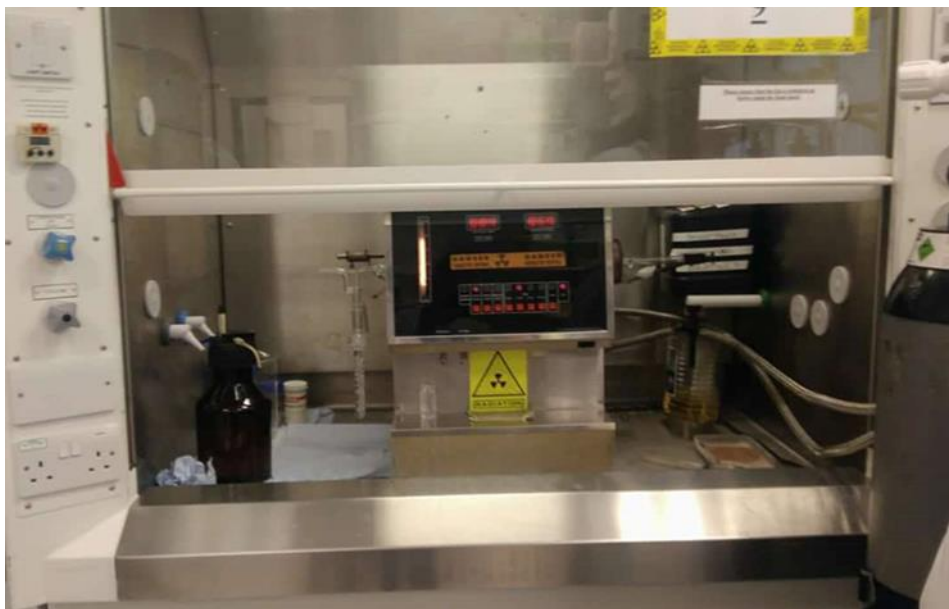
Plate 1: The Harvey Instruments Biological Oxidiser OX400 located in the fume hood located, in the radiation laboratory, which was used to combust the vegetation, soil and hyphae in sand, for all experimental chapters.
