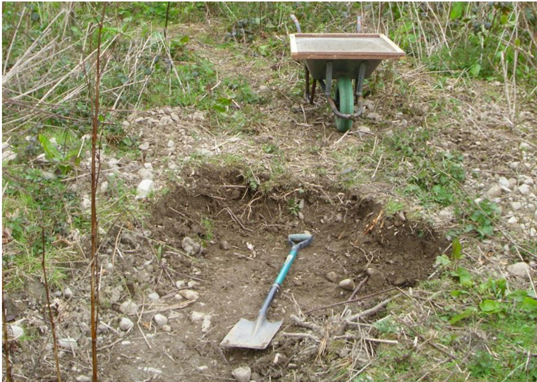
Plate 4: All soil used in the pot experiments was dug from BangorDIVERSE, due to the glacial till nature of the soil we constructed a homemade, wheelbarrow mounted riddle to remove the majority of large stones before air drying the soil in a glasshouse.
