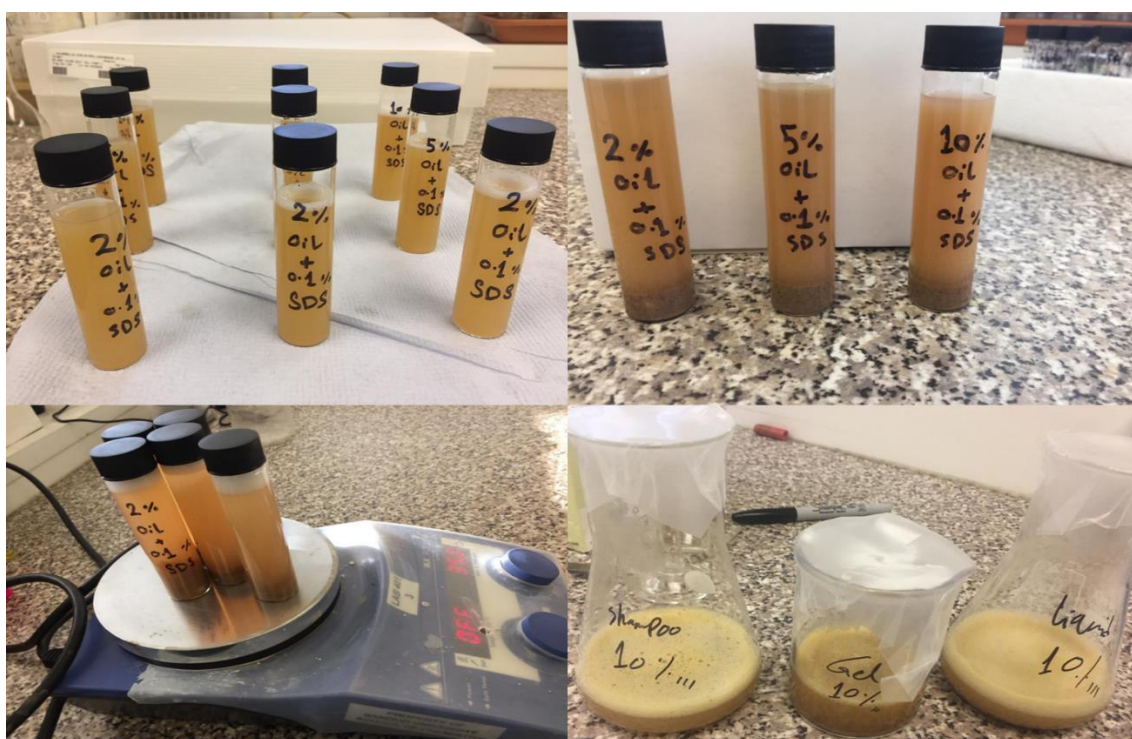
Figure 72 Image of sodium dodecyl sulfate (SDS) and consumer goods (shampoo, shower gel and washing up liquid) solution from contaminated sand during the TPHs recovery experiments.
