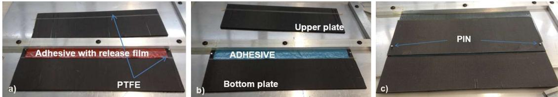
**Figure 3-3 Joint bonded process: a) PTFE tips and film adhesive set up, b) before bonding, c) Final assembly bonded joint**
