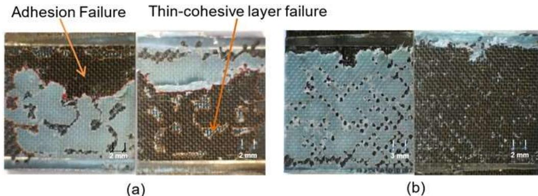
**Figure 4-24 Failure surface SLJ tested under fatigue (a) mode failure typical pattern, (b) failure pattern aged SLJ at 336 cycles**
