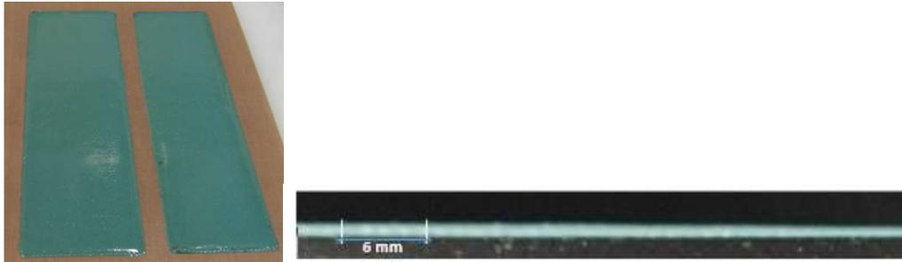
**Figure 3-11 Left Adhesive cured in opened mould, Right side view adhesive cured in open mould**
