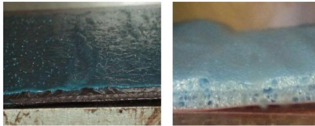
**Figure 3-10 Left adhesive starting to degas. Right adhesive during the degassing process.**
